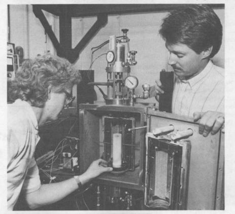
THE HEAT IS ON — or soon will be — for boride samples inside this furnace. Stuart Van Deusen (left) and Terry Aselage (both 1842) are working to produce materials for research that could lead to hightemperature semiconductors; the furnace melts its contents at about 1800°C and lets single crystals form by cooling slowly to about 1000°.
